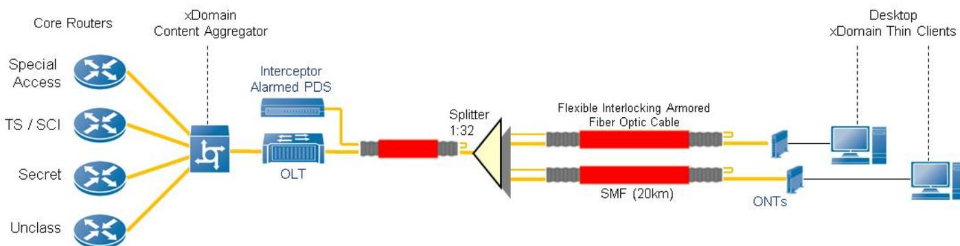
Figure 11: Optical LAN, plus alarmed armored fiber equals All-Secure PON
