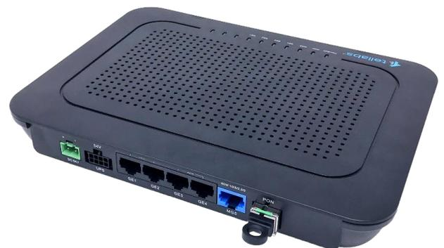
Figure 6: Tellabs FlexSym 205 Optical Network Terminal (ONT205)
