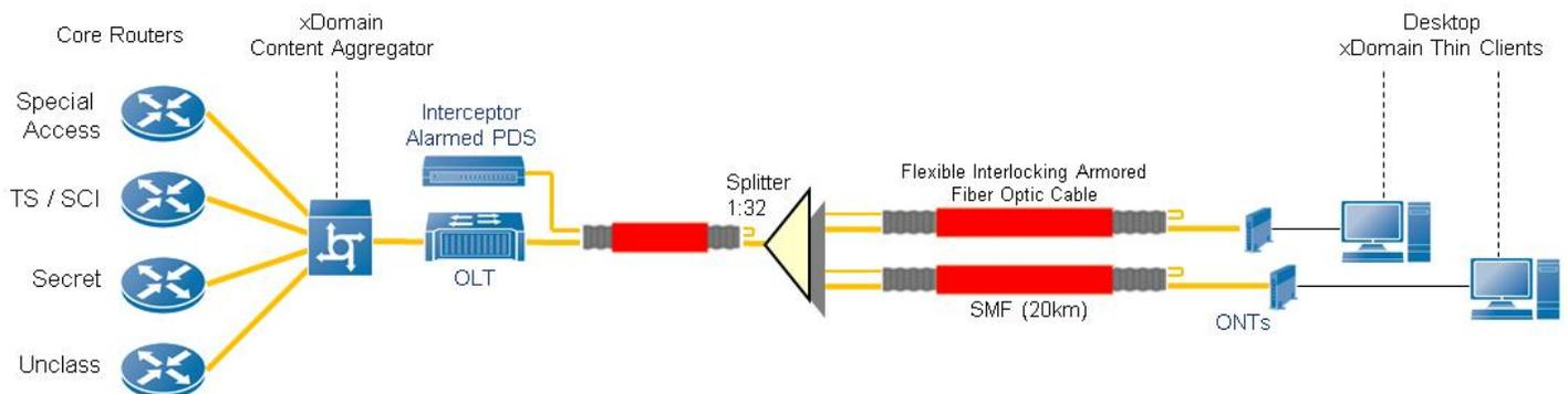
Figure 11: Optical LAN, plus alarmed armored fiber equals All-Secure PON
