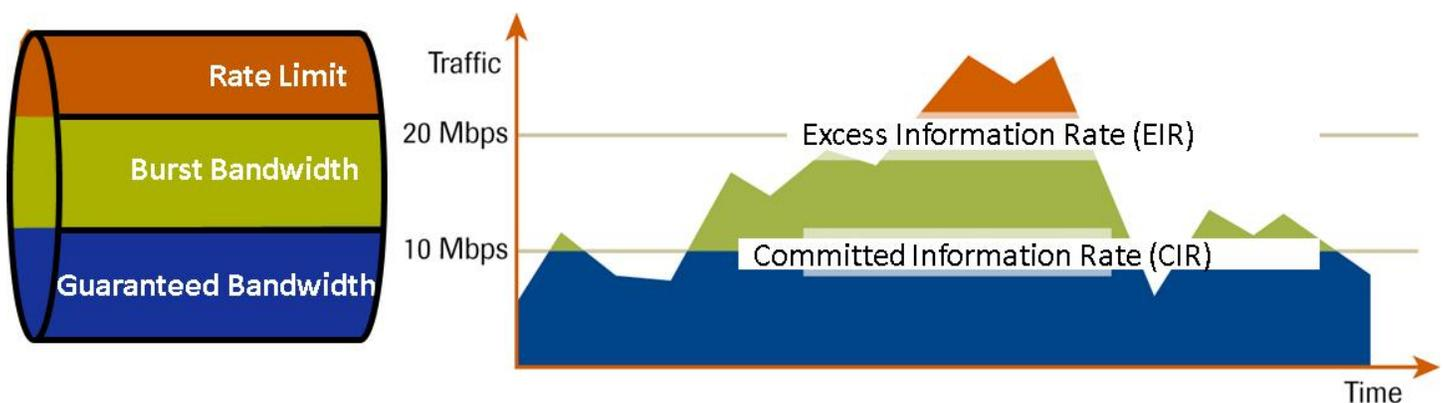
Figure 6: Optical LAN independently set QoS per port and per service, and per up-stream and per downstream
