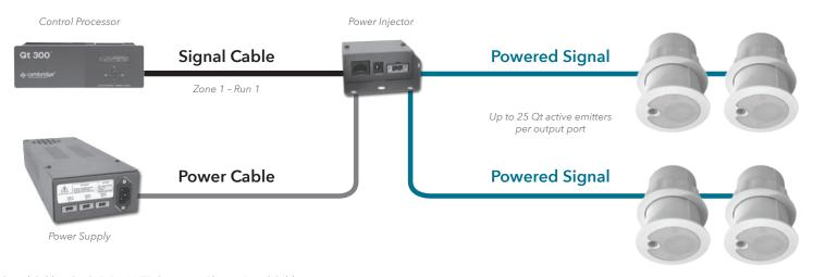
Signal Cable - Cat 3, 5, 5e, 6 UTP Category - Plenum Rated Cable Power Cable - 14/2 Plenum Rated Cable Powered Signal Cable - Cat 3, 5, 5e, 6 UTP Category - Plenum Rated Cable (Active Emitters ship with 16 foot cables)
